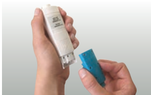
Easy exchange of probes with testo 206-pH1/-pH2/-pH3
