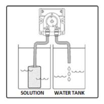
Connect the pump to the timer (or Power Socket 120V AC) The pump will discharge 0,03 cL every 2 seconds.
