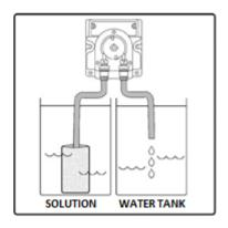
Connect the pump to the timer (or Power Socket 240V AC) The pump will discharge 0,08 cL every 2 seconds.
