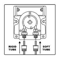
Connect the soft tube to the pump (impulsion – arrow downwards). The injection fitting will be placed at the end of this tube only to inject into a piping. (This fitting has a thread that links it to the piping.)
