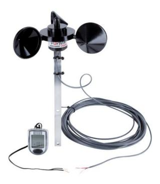
Knowing the wind speed is not only useful - it's informative, it's accurate, and it's fun. The Vortex Pole Mount Anemometer is an inexpensive way to provide you with accurate wind speed in places where AC power may not be available.
