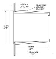
Adjustable location brackets (supplied with the meter) allow the indicator to slide into the cutout and will hold the unit securely in place. 190 mm (7.50") is the minimum amount of room required to install the indicator with the cables connected.
