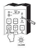
The alarm contacts of **HI 8410** remain closed during normal operation. If the measured <u>conductivity</u> level is not within the tolerance of the set value, the alarm contact will be open.
