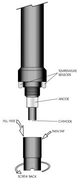
4. With the sensor facing down screw the cap clockwise to the end of the threads. Some electrolyte will overflow.
