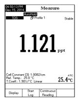
Note: Salinity calibration is made in conductivity mode when using Natural Sea Water or Practical Sea Water measurement. Direct salinity calibration is only possible when using the older percent scale.
