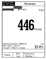
Make sure the TDS factor has been set before taking TDS measurements (see TDS Setup section).
