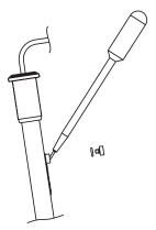
Holding the body of the electrode gently press upper cap with your thumb. This permits the fill solution to drain out of the body. Release cap and verify electrode returns to its original position (you may need to gently assist for this to occur).
