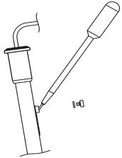
Holding the body of the electrode gently press upper cap with your thumb. This permits the fill solution to drain out of the body. Release cap and verify electrode returns to its original position. (You may need to gently assist for this to occur).
