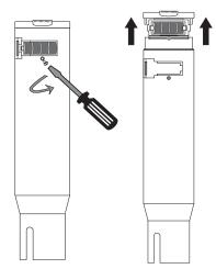
Replace the built-in electrode with a new:
