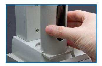
With Clip-Lock  $^{T\!M},$  it only takes a few seconds to exchange the reagent burettes to perform a different titration.
