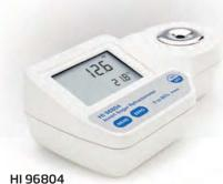
Measures the refractive index to determine the % invert sugar in aqueous solutions. The refractive index of the sample is converted to % by weight concentration units.
