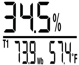
**Note:** If the external Type K probe is not connected, T1-T2, T2-DP, and T2 measurements will not be displayed.
