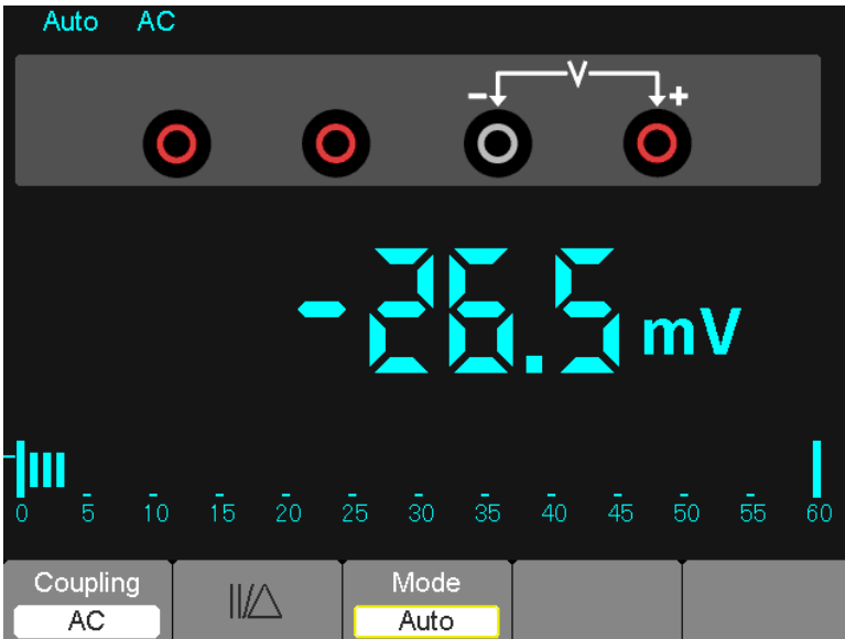
Figure 7-7 AC voltage Measurement
