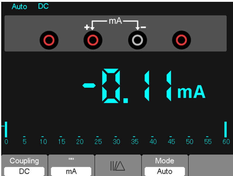
Figure 7-8 DC current Measurement for 600 mA
