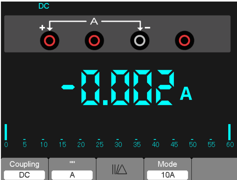
Figure 7-9 DC Current Measurement for 10A
