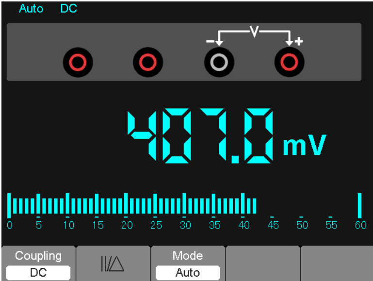
Figure 7-6 DC voltage Measurement
