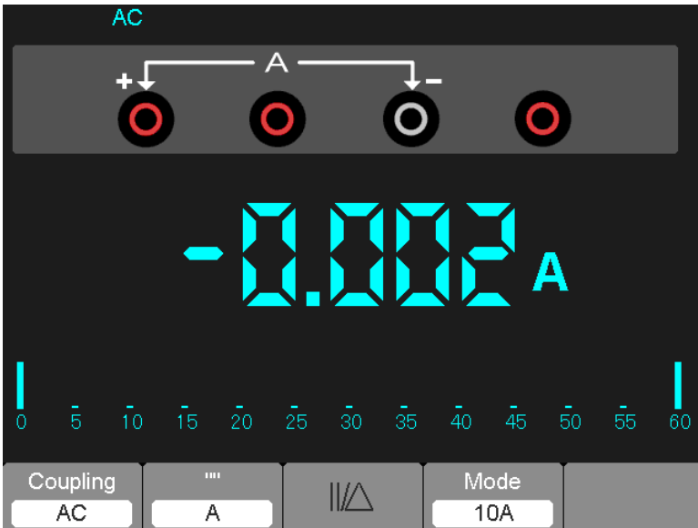
Figure 7-11 AC Current Measurement for 10A
