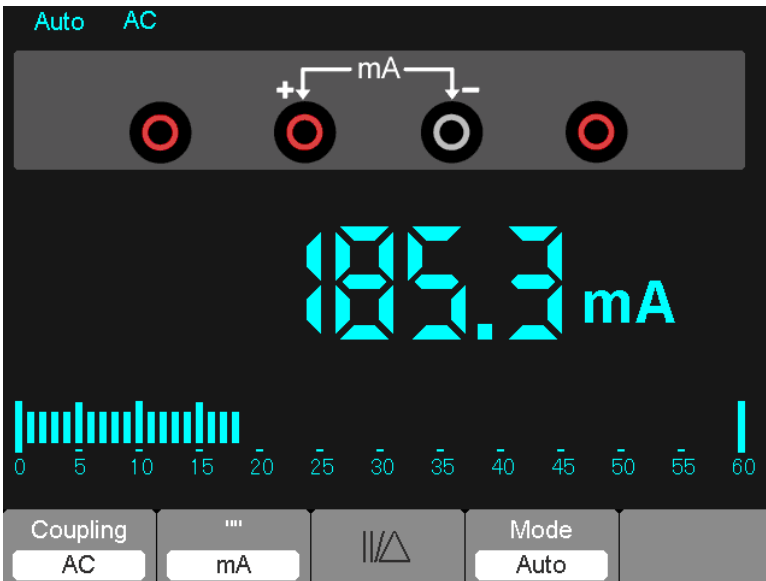
Figure 7-10 AC Current Measurement for 600 mA
