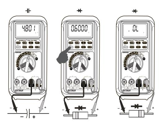
Note: Normal forward voltage drop (forward biased) for a good silicon diode is between 0.400V to 0.900V. A reading higher than that indicates a leaky diode (defective). A zero reading indicates a shorted diode (defective). An OL indicates an open diode (defective). Reverse the test leads connections (reverse biased) across the diode. The digital display shows OL if the diode is good. Any
