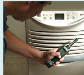
Precision Hygro-Thermometer with 2%RH accuracy and fast 30sec RH response time. Measures Humidity, Temperature, Dew Point, Wet Bulb, GPP and g/kg
